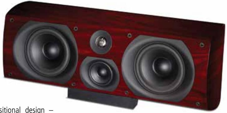
The C3 includes two of the 7" woofers, both active at lower frequencies and with different low pass filter frequencies to maintain proper power response, as well as the same titanium tweeter as the Imagine T3. The specially developed midrange driver is unique to the Imagine C3 and is responsible for the excellent speech articulation of this speaker. The enclosure is rear ported and includes a tuning plug to adjust bass output for different placement options.
